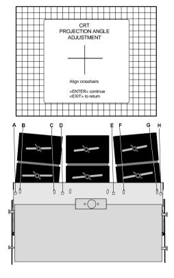
Loosen bolts E, F, G and H to pivot the blue CRT until the center of the Blue image and the center of the Green image coincide. When the angle of the blue CRT is corrected, tighten the four bolts. Press the *<ENTER>* key to continue with the diagonal focusing menu. Press the *<EXIT>* key to return to the CRT projection angle adjustment.
